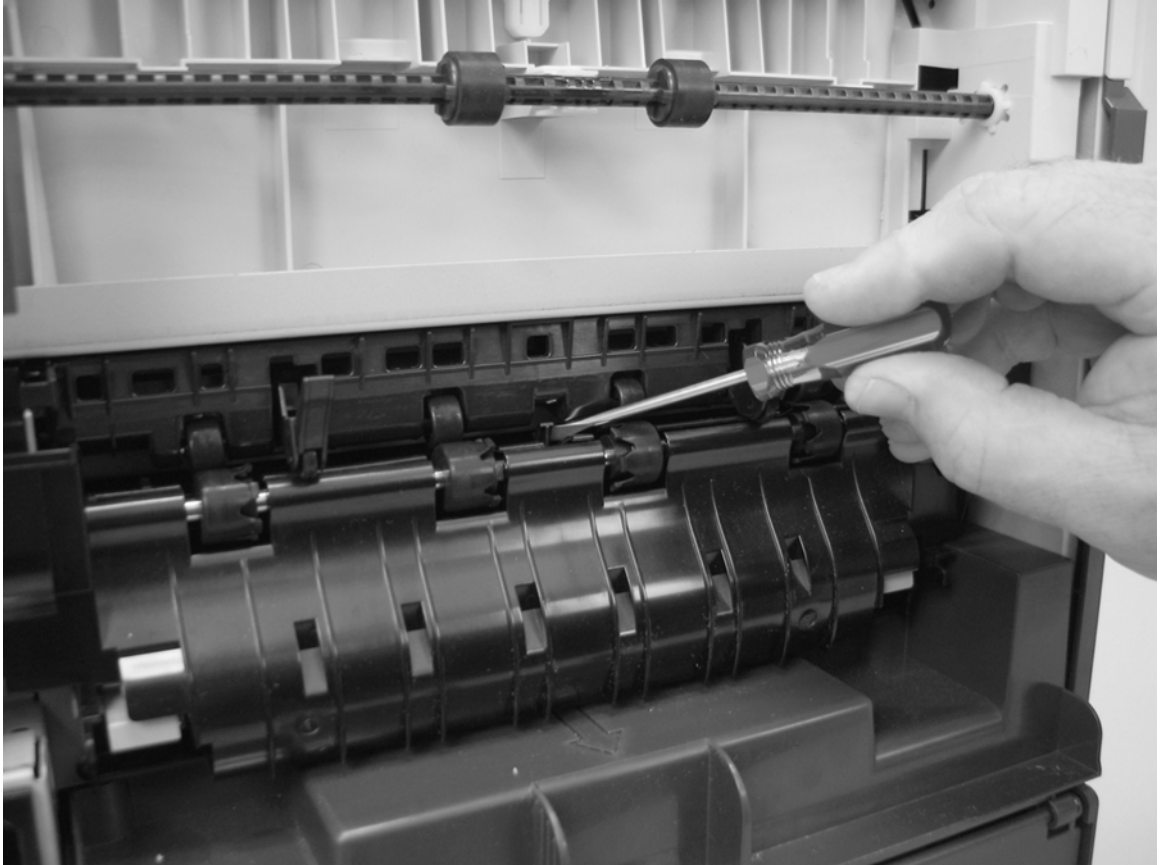
Figure 7-5 Checking the fuser delivery sensor
