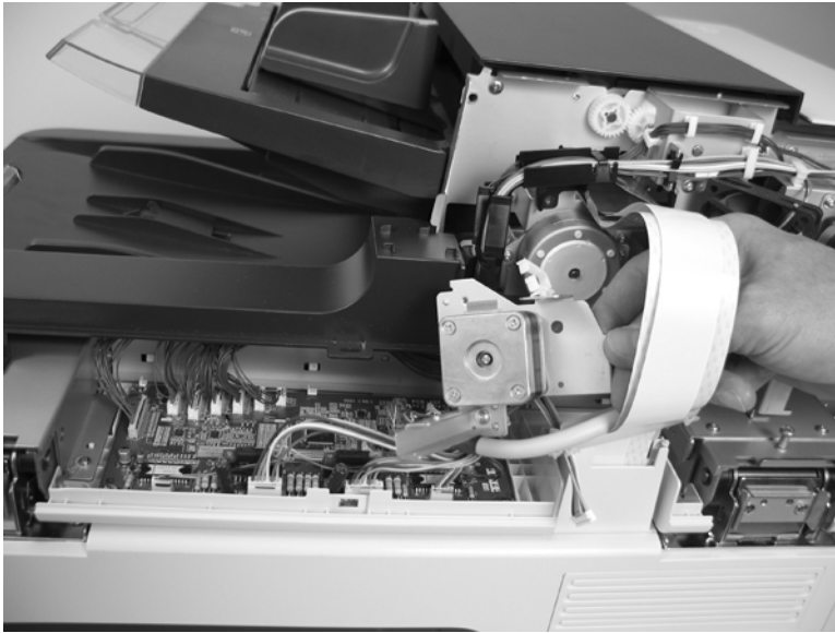
Figure 5-94 Remove the ADF exit-motor assembly (5 of 7)
