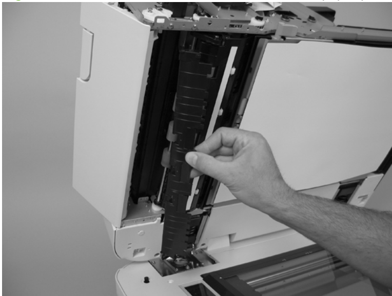
Figure 5-157 Remove the ADF bottom corner inner paper path guide (2 of 2)
