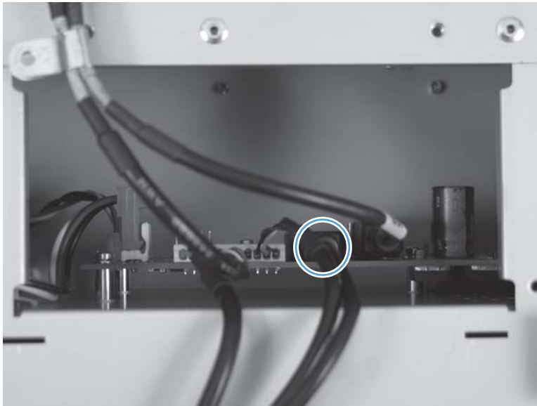
Figure 2-48 Remove the control-panel cable (1 of 3)
