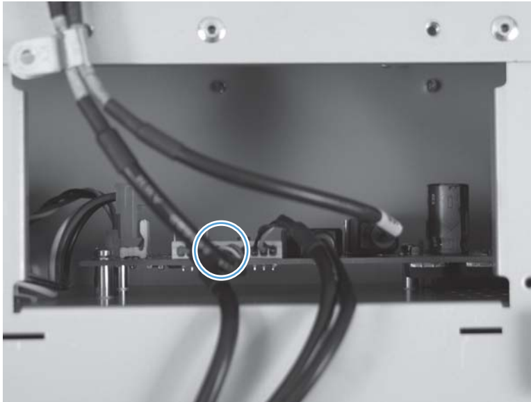
Figure 2-51 Remove the interconnect cable (1 of 4)
