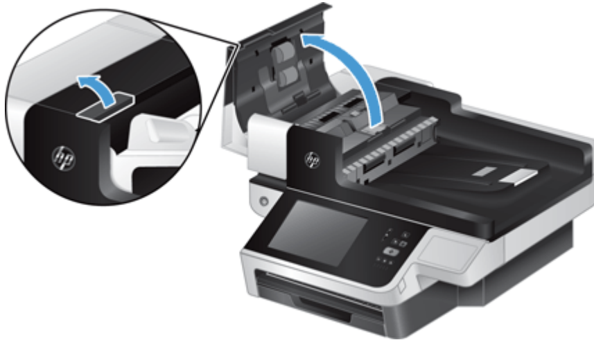
Figure 2-5 Remove the separation pad (1 of 3)
