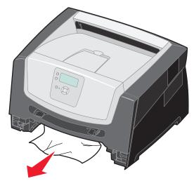
3 Press down on the green duplex flap to release jammed pages from the duplex area.
