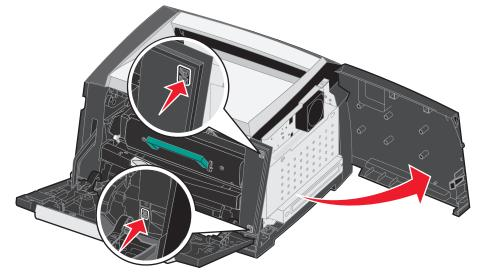
5 Loosen the four screws of the cover to gain access to the system board.
