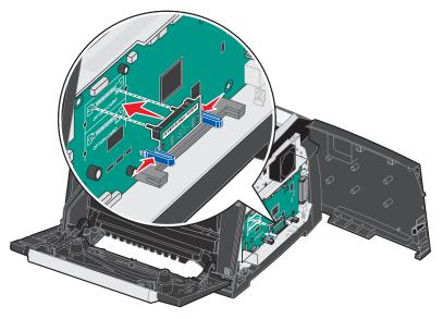
4 Push the flash memory card firmly into the holes of the system board until it *snaps* into place.
