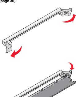
3 Squeeze the retainers, and align the plastic pins on the flash memory card with the holes on the system board.
