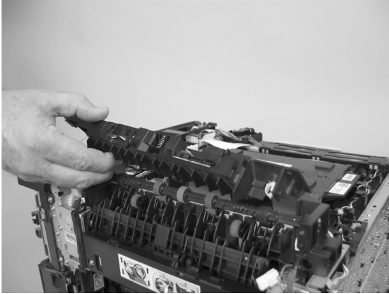
Figure 1-145 Remove the paper-delivery assembly (4 of 4)
