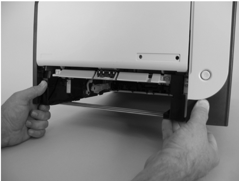
Figure 1-7 Remove the separation roller (1 of 3)
