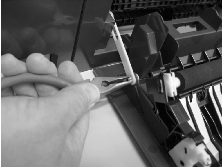
Figure 1-29 Remove the rear door (simplex product) (1 of 4)
