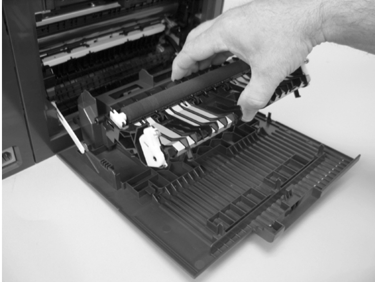
Figure 1-68 Remove the feed assembly (2 of 2)
