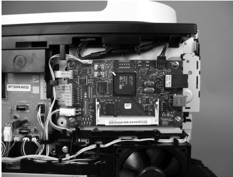
Figure 1-107 Remove the formatter PCA (1 of 2)
