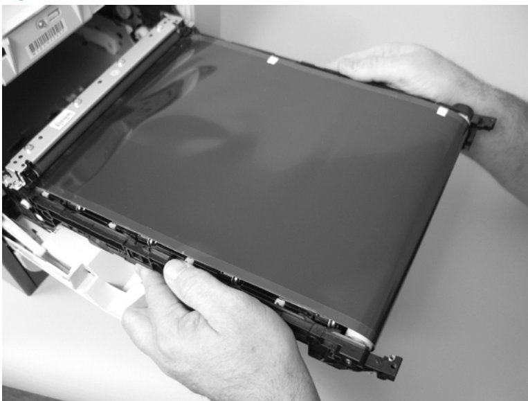
Figure 1-97 Remove the ITB (6 of 6)
