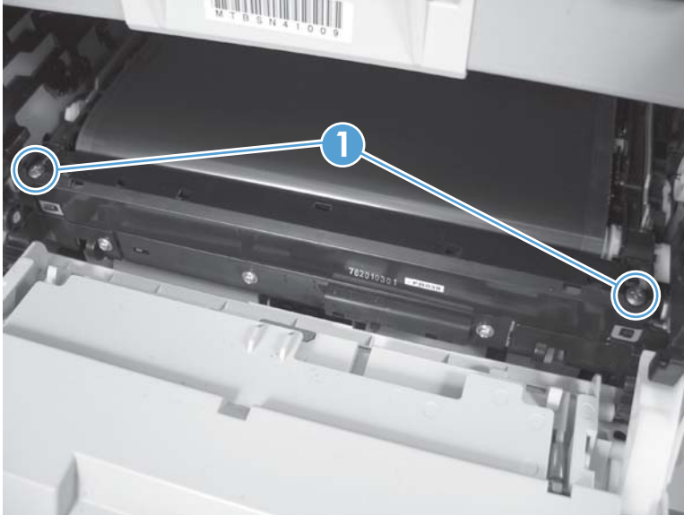
Figure 1-92 Remove the ITB (1 of 6)
