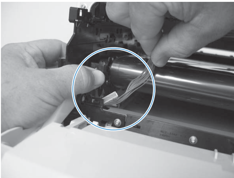
Figure 1-125 Reinstall the color-misregistration sensor assembly PCA (1 of 2)
