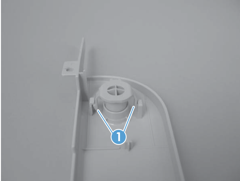
Figure 1-66 Remove the right-front cover and power button (2 of 2)
