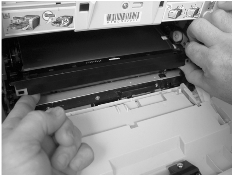
Figure 1-95 Remove the ITB (4 of 6)
