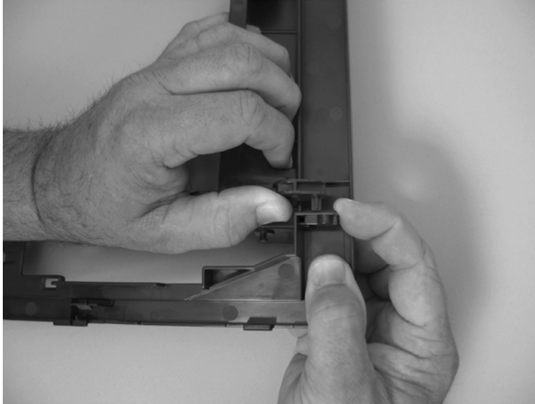
Figure 1-41 Remove the rear cover and feed guide (simplex product) (5 of 6)
