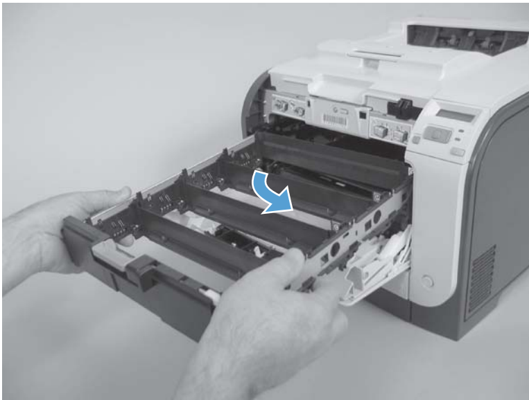
Figure 1-16 Remove the print-cartridge drawer (2 of 3)
