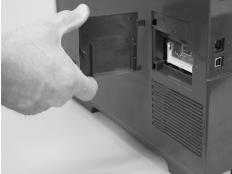
Figure 1-18 Remove the DIMM cover
