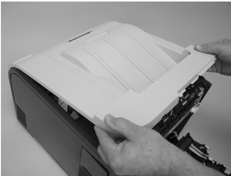
Figure 1-57 Remove the upper-cover assembly (4 of 4)
