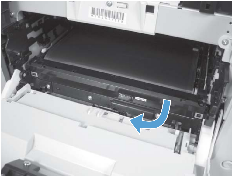
Figure 1-93 Remove the ITB (2 of 6)
