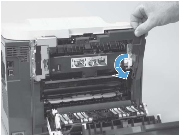
Figure 1-26 Remove the rear-upper cover (2 of 2)
