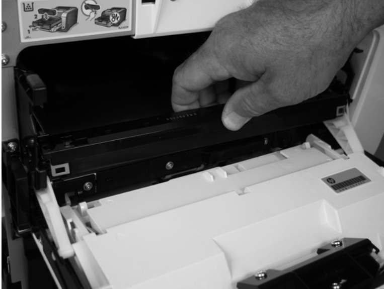
Figure 1-124 Remove the color-misregistration sensor assembly PCA (4 of 4)
