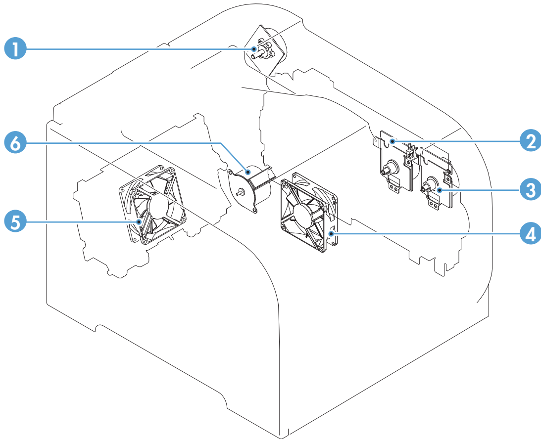
Figure 2-6 Motors and fans
